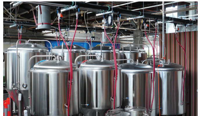
COOL-FIT fabricated T90 with brass 1" thread connection allows for direct connection of hoses to fermentation tanks
