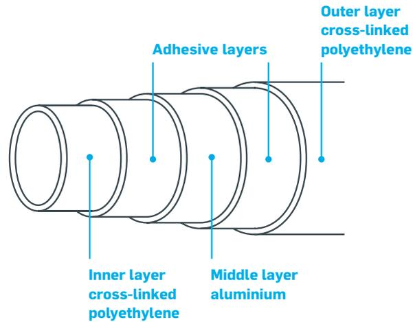
Duopex Water uses the multilayer pipe system for potable hot and cold-water applications. Available in 16-63 mm diameters, it's made to handle the big stuff. And when combined with our DR brass fittings and stainless steel crimp ring it's also quicker and easier than other systems.
