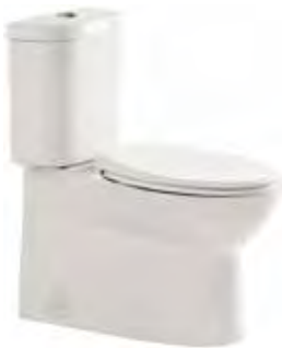
Studio Close coupled back to wall toilet suite Soft close, quick release seat WELS 4 star, 4.5/3 ltr/flush Average flush: 3.5 litres S Trap: 140mm-270mm (180mm recommended) P Trap: 190mm Back and bottom inlet available
