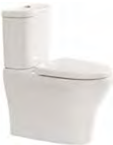
Cygnet Overheight close coupled back to wall toilet suite WELS 4 star, 4.5/3 ltr/flush Average flush: 3.5 litres Soft close seat Raised pan height S Trap: 140mm-250mm (180mm recommended) P Trap: 190mm Bottom and back inlet available Raised height pan Ambulant compliant
