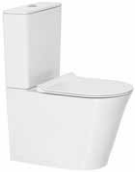
Heron Hygiene Rim Close Coupled Back to Wall Toilet Suite Soft close, quick release seat WELS 4 star, 4.5/3 ltr/flush Average Flush: 3.5 ltrs S Trap : 90-140mm P Trap : 180mm Bottom inlet Back and Bottom inlet available
