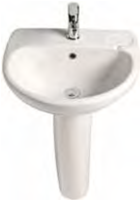
Studio Wall Basin 500 500mm x 425mm 1 or 3 tapholes Overflow Optional pedestal available Wall brackets included
