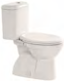
Heron Close coupled square toilet suite Soft close, quick release seat WELS 4 star, 4.5/3 ltr/flush Average flush : 3.5 ltrs S Trap : 140mm P Trap : 185mm Bottom inlet 20mm pan collar available to achieve S trap set out of 120-160mm
