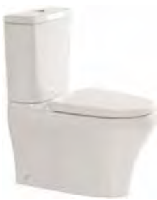
Cygnet Close coupled back to wall toilet suite Soft close, quick release seat WELS 4 star, 4.5/3 ltr/flush Average flush: 3.5 litres S Trap: 140mm-270mm (180mm recommended) P Trap: 190mm Back and bottom inlet available
