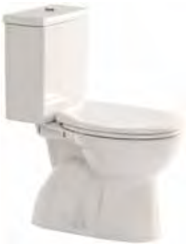
Heron Close coupled square toilet suite Soft close, quick release seat WELS 4 star, 4.5/3 ltr/flush Average flush : 3.5 ltrs S Trap : 140mm P Trap : 185mm Bottom inlet 20mm pan collar available to achieve S trap set out of 120-160mm
