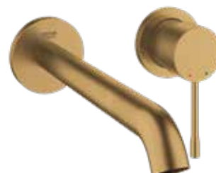
19 967 EN1 + 32 635 000 19 967 A01 + 32 635 000 19 967 GN1 + 32 635 000 Essence Wall mounted basin mixer set +separate concealed body Projection 230mm WELS 5 star, 6ltrs/min ** Also available as wall mounted bath mixer set
