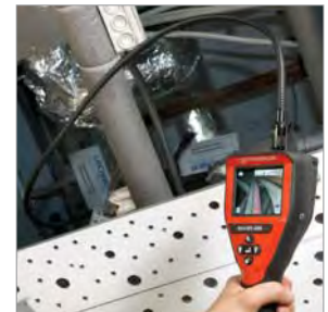
Camera head with high-performance LEDs
