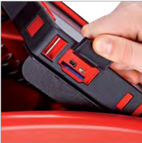
Cover protected connections for SD-card, Micro-HDMI, Mini-USB
