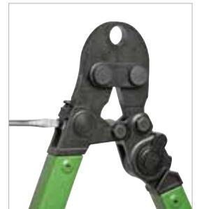
If the gauge fails, repeat adjustment until trial crimped joint is correct. More detailed instructions are included with the tool.
