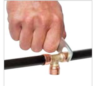
If the gauge experiences any interference the joint is under crimped. The tool should then be adjusted. (See adjustment instructions in this manual). **Do not double crimp.**
