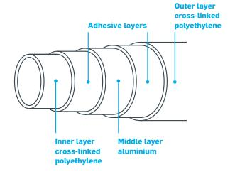
Duopex Water uses the multilayer pipe system for potable hot and cold-water applications. Available in 16-63 mm diameters, it's made to handle the big stuff. And when combined with our DR brass fittings and stainless steel crimp ring it's also quicker and easier than other systems.
