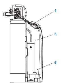
Refill the unit in such a way that no dirt can get into the storage area (5) (if necessary, clean the pakkages containing the regenerative before use).
