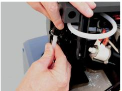
Run the the brine hose from the inside through the bore to the outside and insert it as far as it will go (a depth of about 15 mm) in the elbow.
