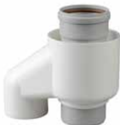
FLU ADAPTOR - TWIN TO COAX Thermann Part # 9507662 CF32C002 This component is required with wall and roof terminals in case of room sealed installation.
