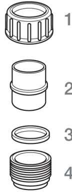
Figure 34: Screw-threaded joint with flange bushing (available \varnothing 40–110 mm)
